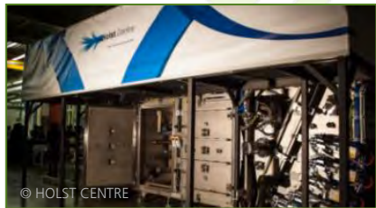
R2R equipment for manufacturing ultra-barrier webs ( \text{WVTR}: 10^{-6} \text{ g m}^{-2} \text{ d}^{-1} ) for organic electronics (Holst Centre)
