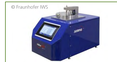
Measurement of barrier webs for organic flexible electronics with \text{WVTR} up to 10^{-6} \text{ g m}^{-2} \text{ d}^{-1}
