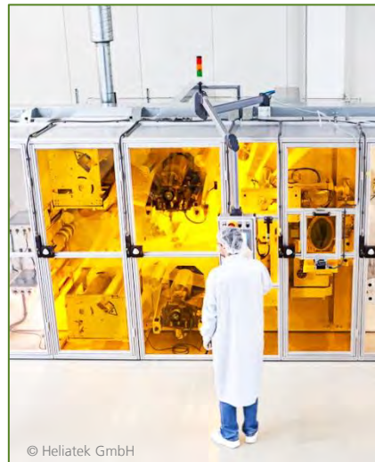
R2R production of HeliaFilm® (Heliatek GmbH)
