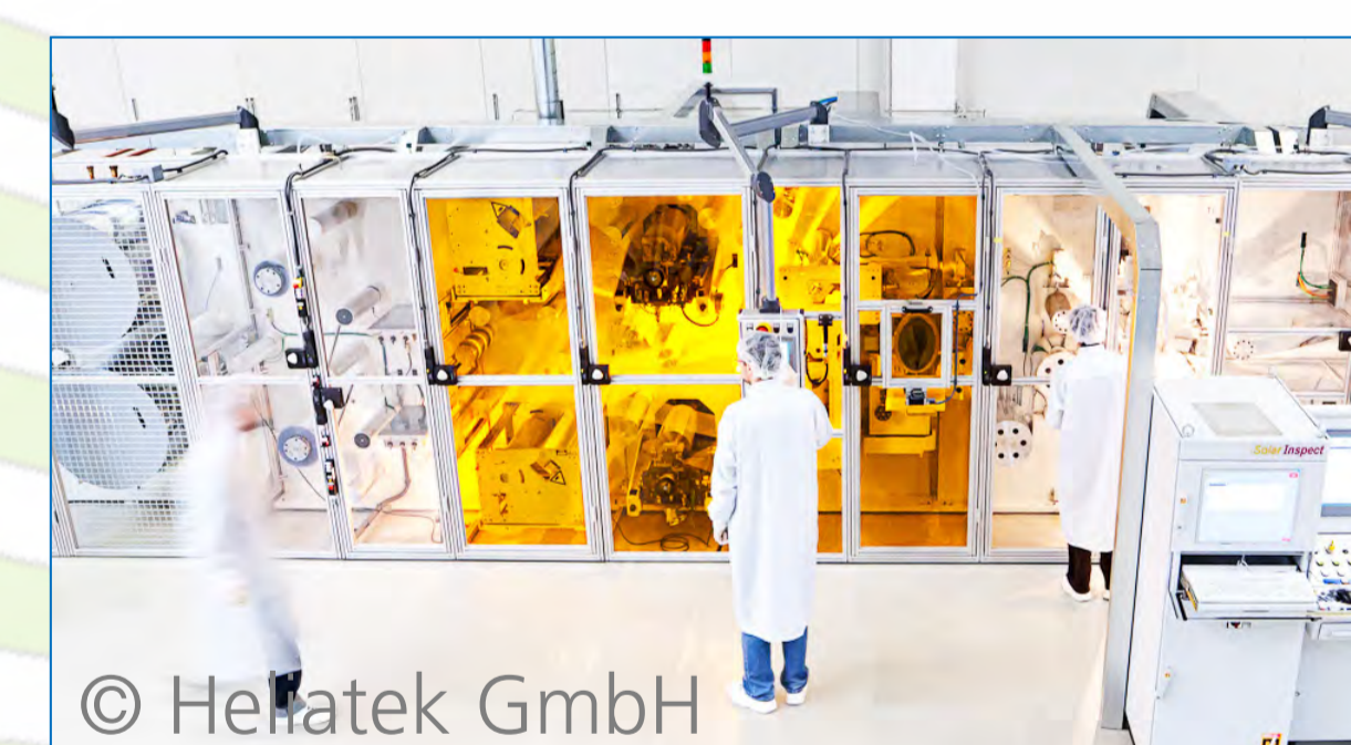
R2R production of HeliaFilm® (Heliatek GmbH)
